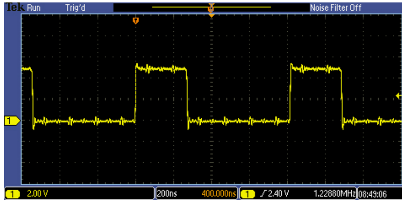
Figure 8: Scope display of the fast oscillation output
