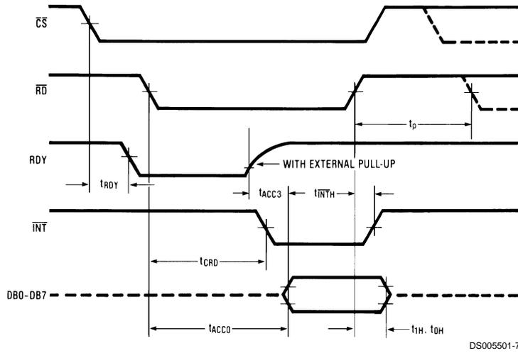
**Note:** On power-up the state of  $\overline{\text{INT}}$  can be high or low.
