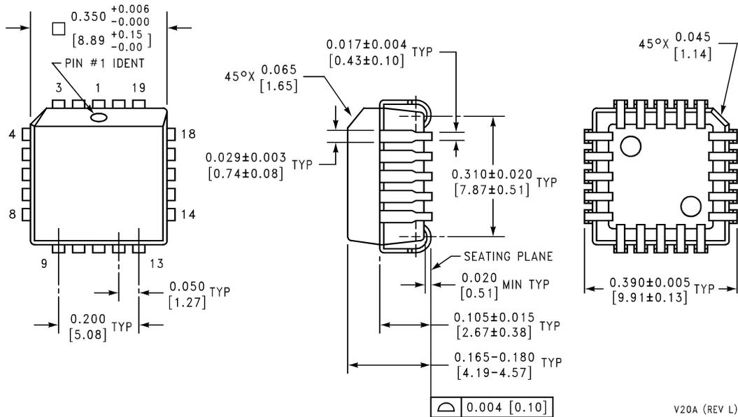
**Molded Chip Carrier Package (V)**
