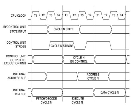
Figure 2-9. Control Unit Timing
