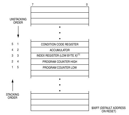
1. High byte (H) of index register is not stacked.
