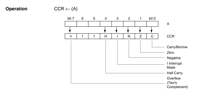
**Description** Transfers the contents of A to the condition code register (CCR). The contents of A are unchanged. If this instruction causes the I bit to change from 0 to 1, a one bus cycle delay is imposed before interrupts become masked. This assures that the next instruction after a TAP instruction will always be executed even if an interrupt became pending during the TAP instruction.
