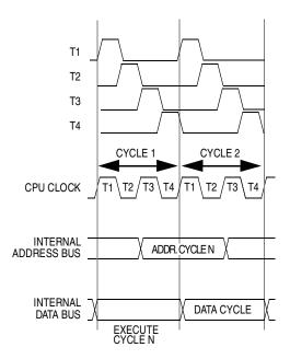
Figure 2-8. Internal Timing Detail
