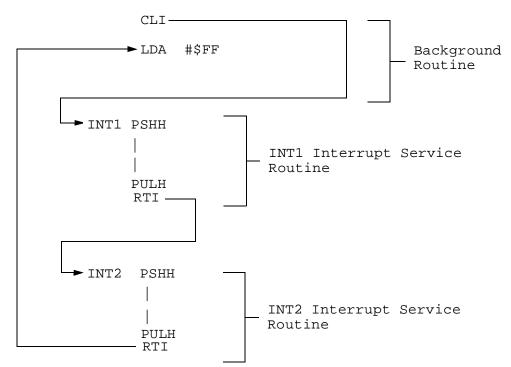
Figure 3-5. Interrupt Recognition Example 2
