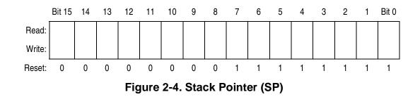
**NOTE:** Although preset to \$00FF, the location of the stack is arbitrary and may be relocated by the user to anywhere that random-access memory (RAM) resides within the memory map. Moving the SP out of page 0 (\$0000 to \$00FF) will free up address space, which may be accessed using the efficient direct addressing mode.
