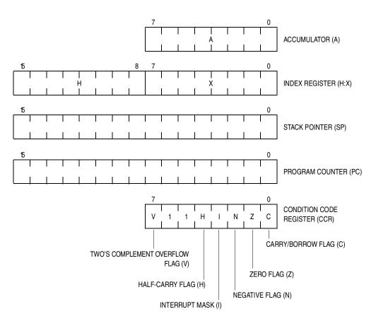
Figure 2-1. CPU08 Programming Model
